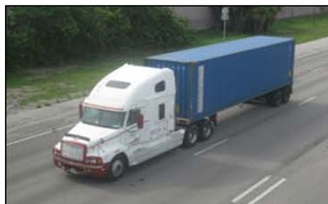
Tractor with Attached Chassie-Carrier
